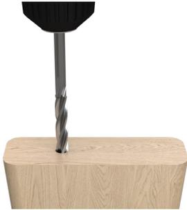
1. Drill two holes straight into the leg
